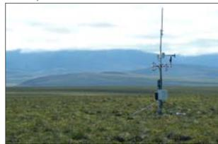
USGS stations collect data on climate conditions, radiation balance, active layer and permafrost temperature. Collected data are transmitted in real time. (photo: Station U31: Marsh Creek)
