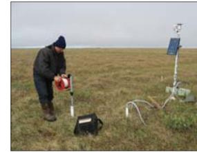
Measurements of ground temperature boreholes help us to understand long-term reaction of permafrost to climate change (Photo: UAF TSP borehole at Deadhorse).
