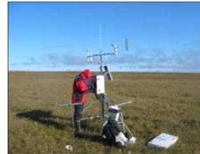
Several NRC soil climate research stations on the North Slope provide data on near-surface ground temperature and climate conditions to help us understand short-term changes in active-layer-permafrost system (photo: NRC West Dock 1 station).
